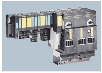
The Failsafe motor starter has been developed on the basis of the High-Feature motor starter. It differs in that, in addition to a motor starter protector and contactor assembly, a safe solidstate evaluation circuit is installed for error detection purposes which makes the motor starter failsafe.
