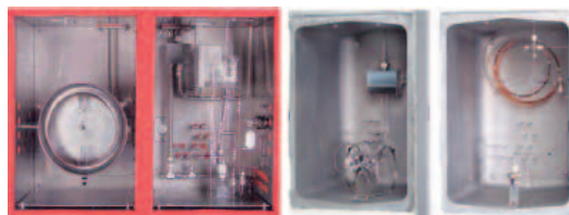
Fig. 11: MAXUM Dual oven concept Left: split air bath, temperature programmed Right: dual airless
