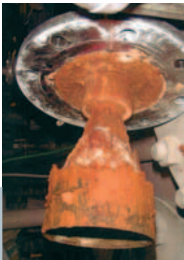
Installed in an application for the production of titanium dioxide, the pulse radar delivers reliable measurement results despite extreme deposits at the horn antenna
