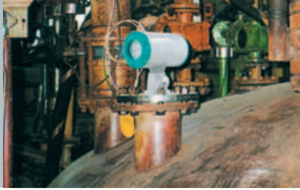
Level measurement of dyes: Application of a SITRANS LR 300 with non-contact radar technology
