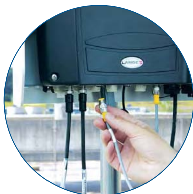
New sensors are recognised automatically.
