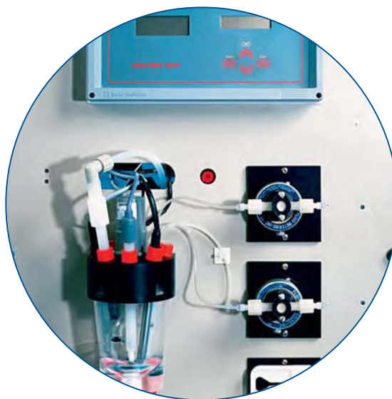
Analysis unit of the 8810 analyser, with automatic electrode cleaning
