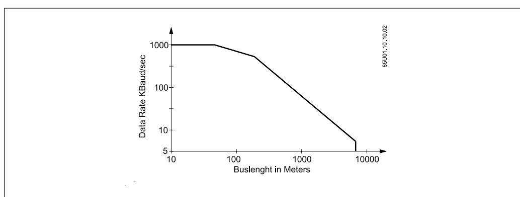
At 1000 kB transmission rate the 40 m cable length cannot be guaranteed in all cases. For each system the transmission delay in receiver/transmitter has to be evaluated for a correct function of the system.
