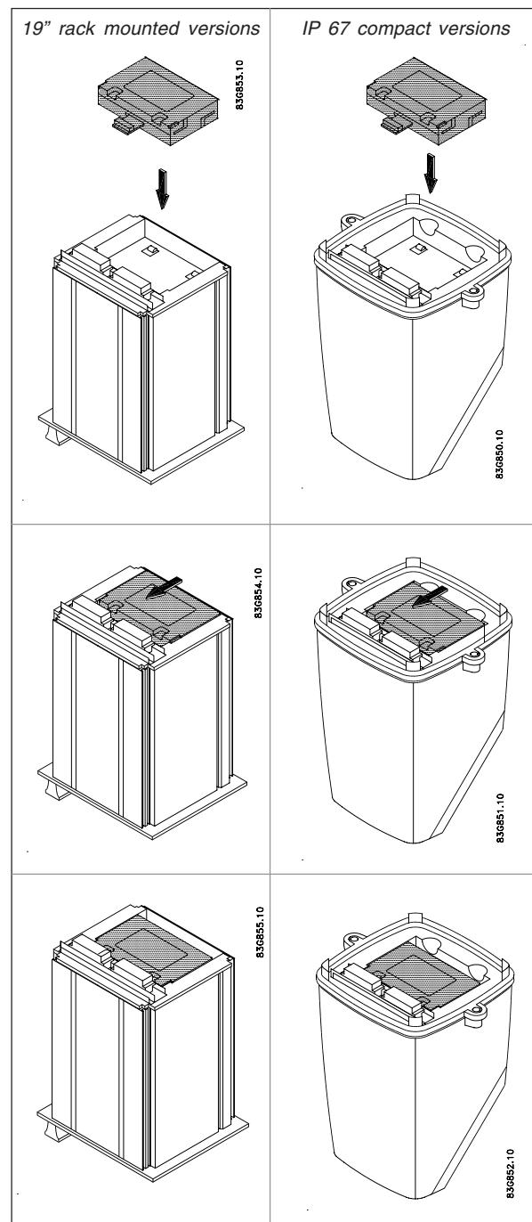
1. Unpack the add-on module and insert it in the bottom of the signal converter as shown.
