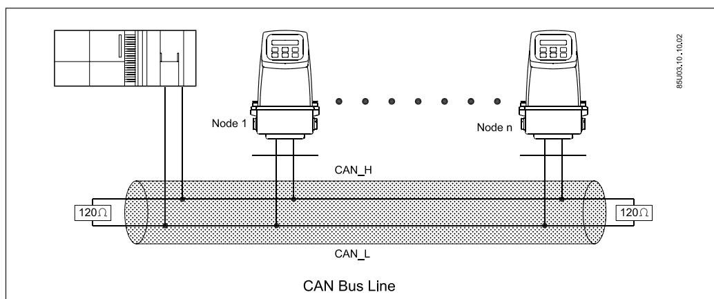
A CAN system must always be terminated correctly. Two termination resistors must be present, one in each end of the trunk line.
