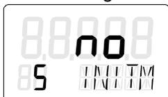
5. Start the initialization process. Press the increment button  $\triangle$  for at least 5 seconds until the digital display shows the following:
