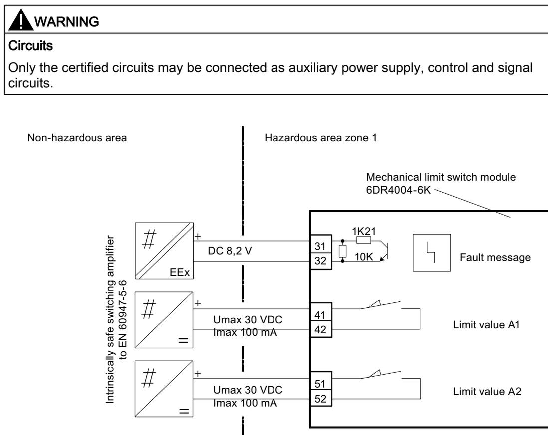
Figure 6-17 Mechanical limit switch module 6DR4004-6K, Ex i
