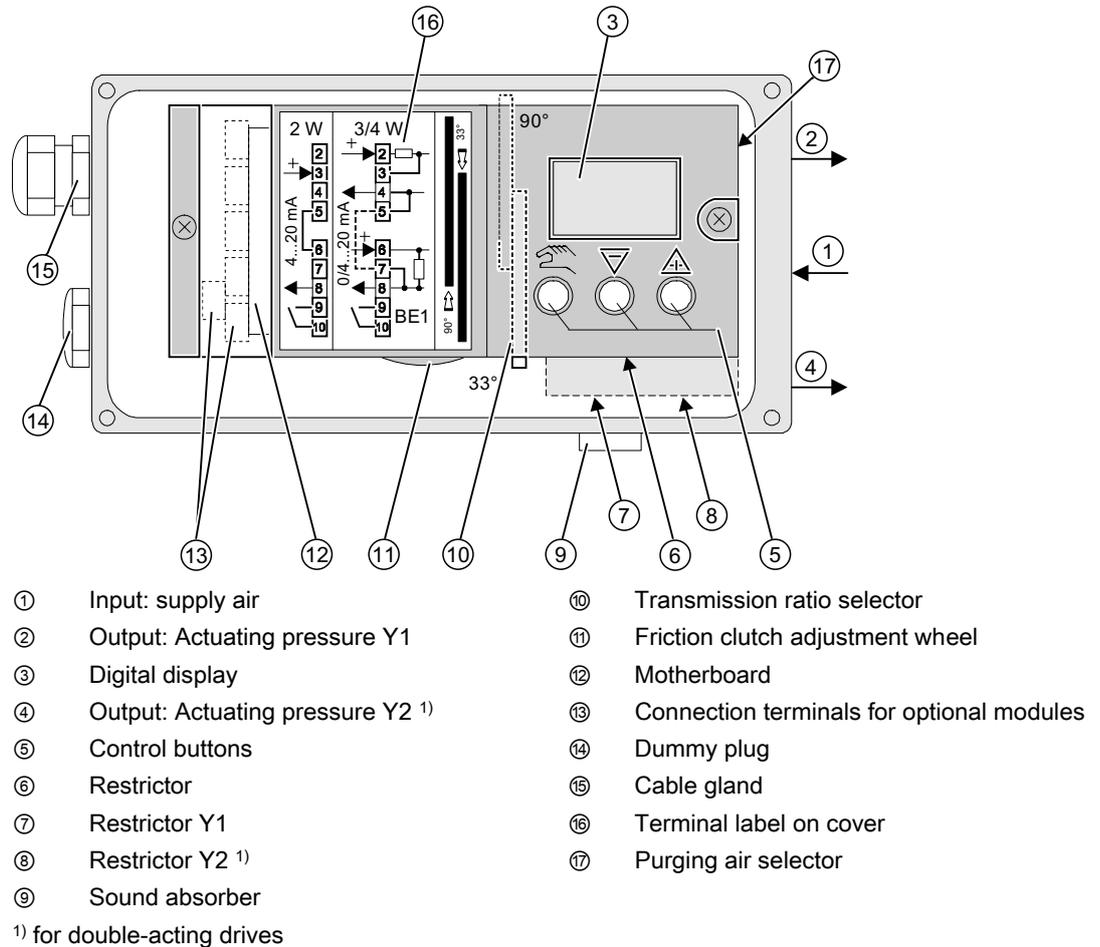
Figure 3-6 View of basic positioner with cover open
