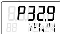
7. Determine the end position 1 of the actuator.
