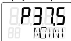
2. Check whether the mechanical unit can be moved freely in the entire actuating range. For this purpose, move the actuator to the top and the bottom end positions alternately using the  $\triangle$  increment or the  $\nabla$  decrement buttons.
