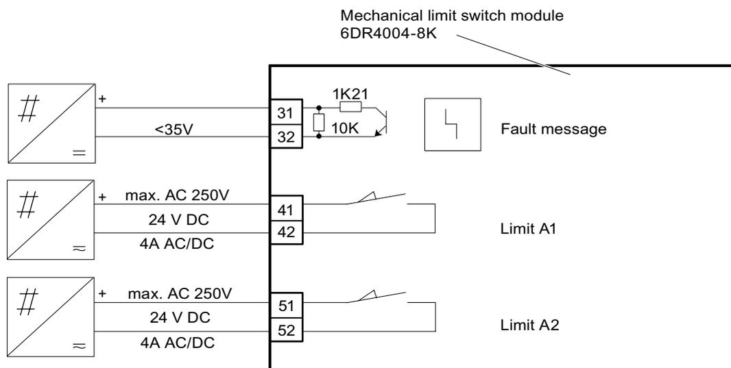
Figure 6-8 Mechanical limit switch module 6DR4004-8K, not Ex
