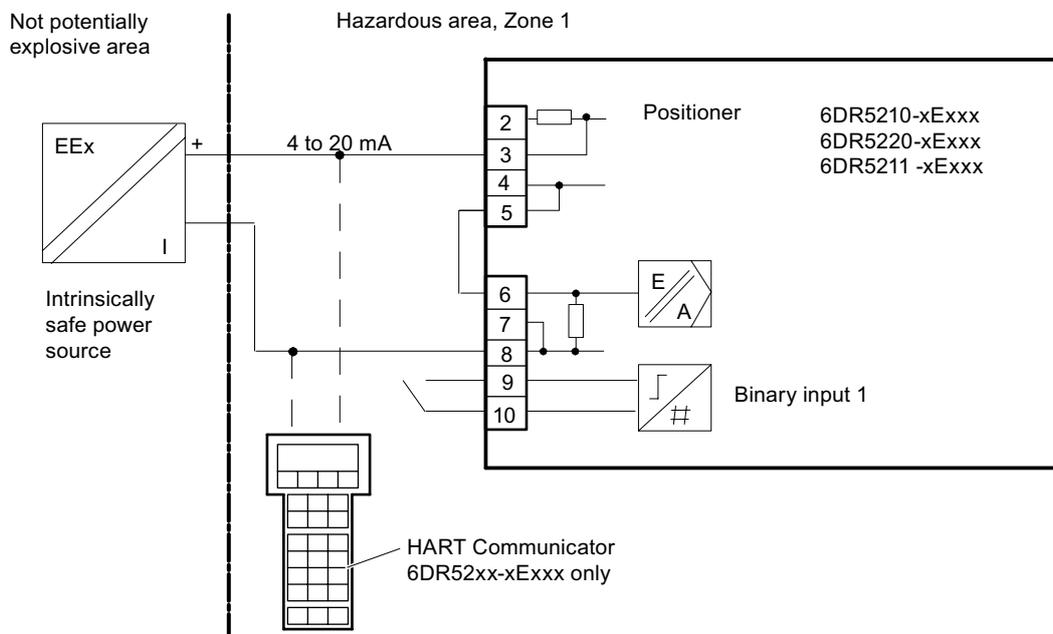
Figure 6-11 Two-wire connection, Ex i
