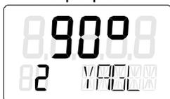
4. Call the "INITM" parameter. Press the
