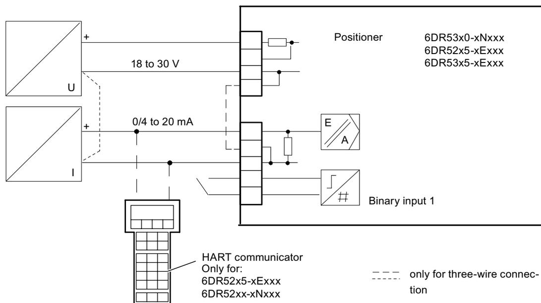
Figure 6-4 Three/four-wire connection
