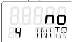
5. Start the initialization process. To do this, press the increment button
