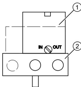
Figure 3-13 Purge air switch on the pneumatic block; view of the positioner on the pneumatic connection side when the cover is open
