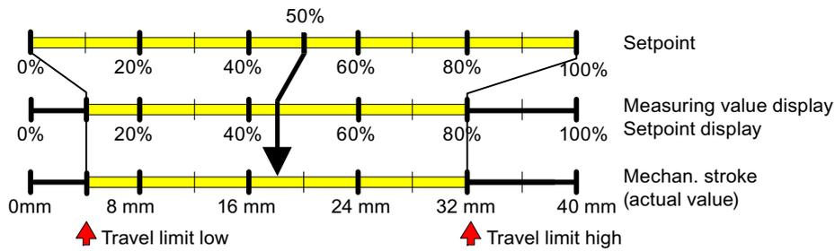
Figure 10-4 Example: YNRM = MPOS with YA = 10 % and YE = 80 %
