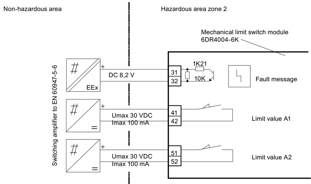
Figure 6-25 Mechanical limit switch module 6DR4004-6K, Ex n
