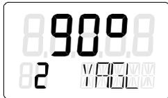
4. Call the fourth parameter "INITA". Press the
