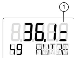
Figure 10-7 Display of a threshold 2 error message
