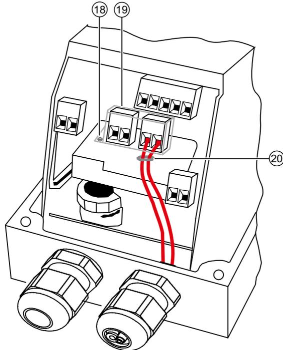
Figure 6-18 Connecting the cables
