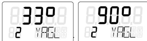
3. Check whether the value displayed in the "YAGL" parameter matches the setting of the transmission ratio selector. If required, change the setting of the transmission ratio selector to 33° or 90°.
