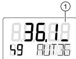
Figure 10-6 Display of a threshold 1 error message
