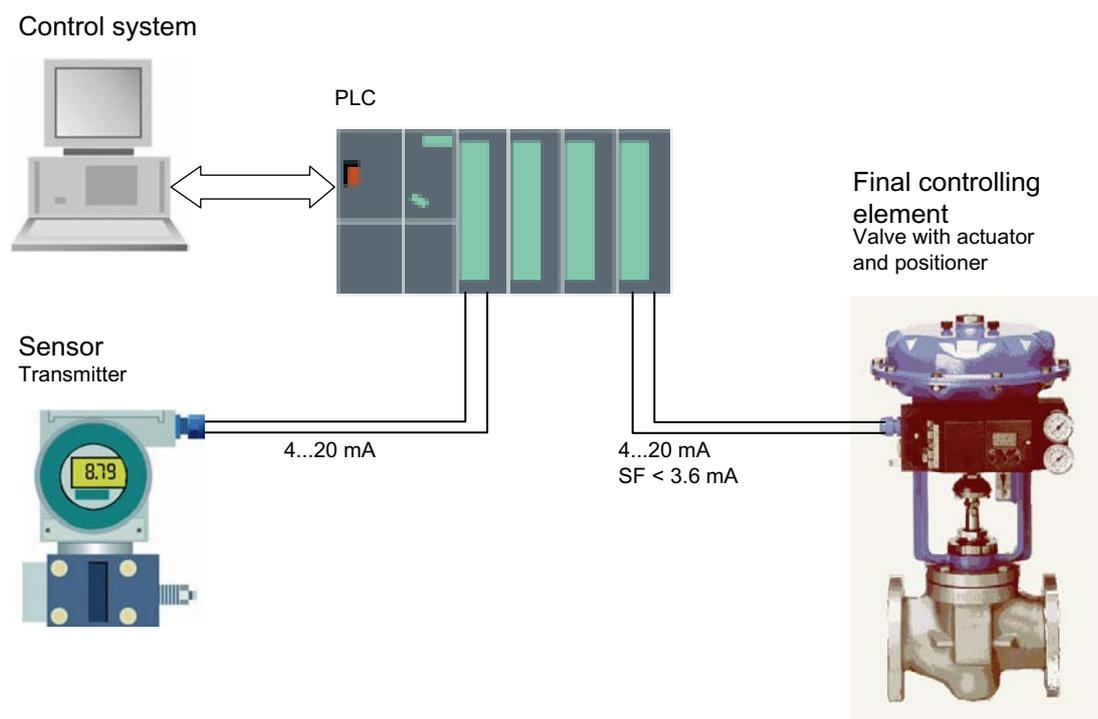
S<sub>F</sub> Failure signal
