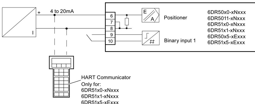
Figure 6-2 Two-wire connection
