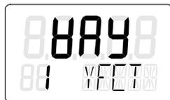
2. Call the second parameter "YAGL". Press the
