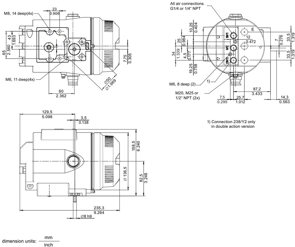
Figure 14-4 Dimensions of device version with flameproof metal housing
