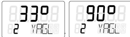
3. Check whether the value displayed in the "YAGL" parameter matches with the setting of the transmission ratio selector. If required, change the setting of the transmission ratio selector to 33° or 90°.
