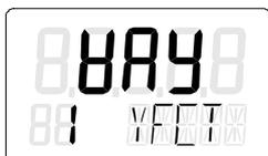
2. Set the "YFCT" parameter to "turn". Press the
