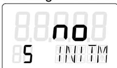
6. Start the initialization process. To do this, press the increment button  $\triangle$  for at least 5 seconds until the digital display shows the following:
