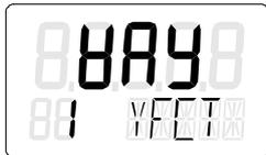
2. Change the actuator type from linear to the part-turn actuator. Change the parameter setting using the ▾ decrement button. The following is shown on the digital display:
