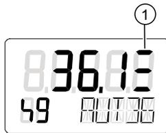
Figure 10-8 Display of a threshold 3 error message
