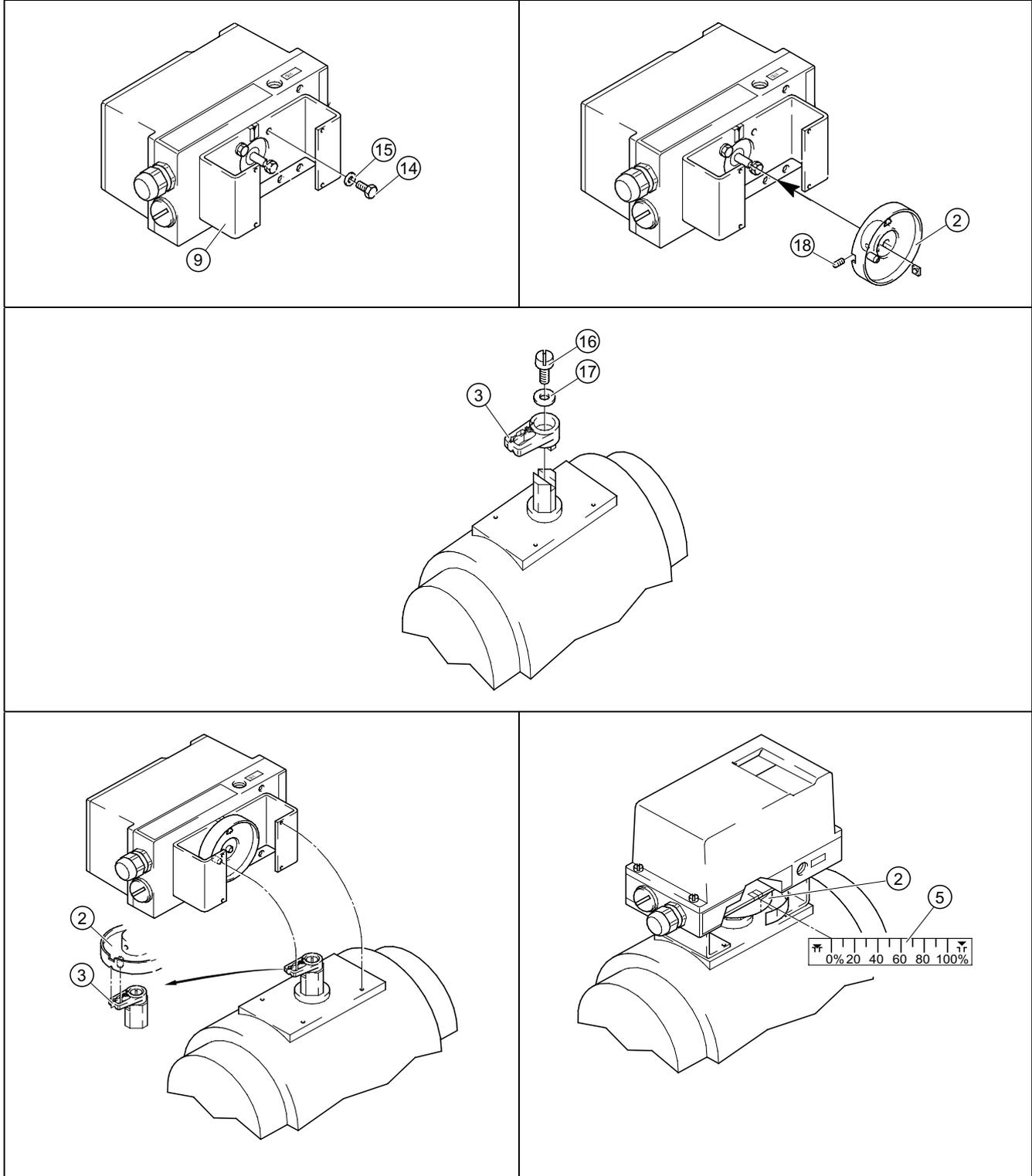
Assembly procedure for the positioner with part-turn actuator and flameproof enclosure
