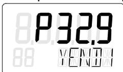
8. Determine the end position 1 of the actuator spindle. Move the actuator spindle to the desired position by pressing the  $\triangle$  increment or  $\nabla$  decrement buttons. Accept the current position of the actuator spindle by pressing the  $\square$  operating mode button. The following is shown on the digital display:
