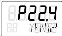
Now move the actuator to the position which you want to define as the second end position with the increment  $\Delta$  and decrement  $\nabla$  key. Then press the operation mode key  $\square$ . This enters the current position as end position 2.
