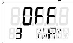
You only need to set this parameter if you want to have the total stroke in mm displayed at the end of the initialization phase. To do this, select the same value in the display to which you have set the carrier pin to the scale on the lever.
