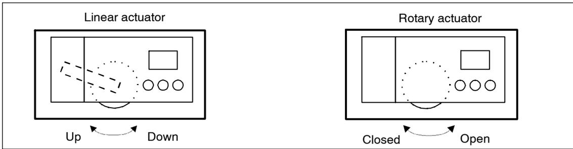
Figure 3-26 Direction of action of the actuators
