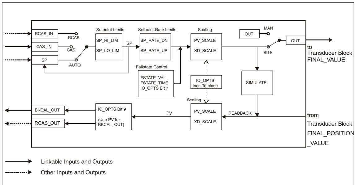
Figure 5-2 Function schematic of AO function block
