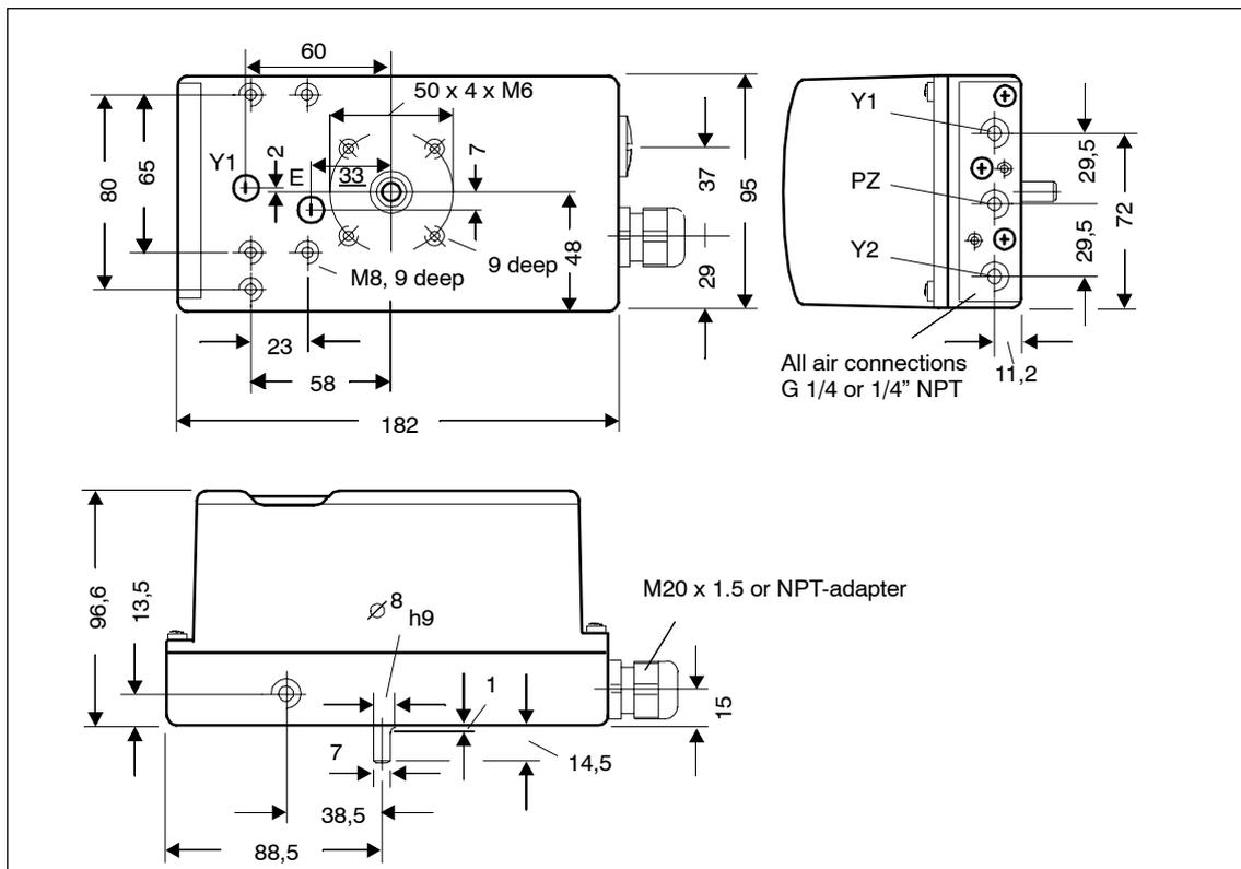
Figure 3-1 Dimensional drawing version plastic housing 6DR5xx0
