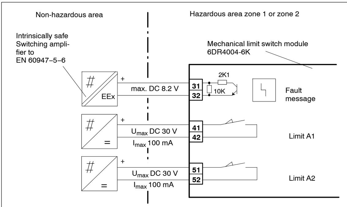
Figure 3-25 Mechanical limit switch module 6DR4004-6K, EEx i
