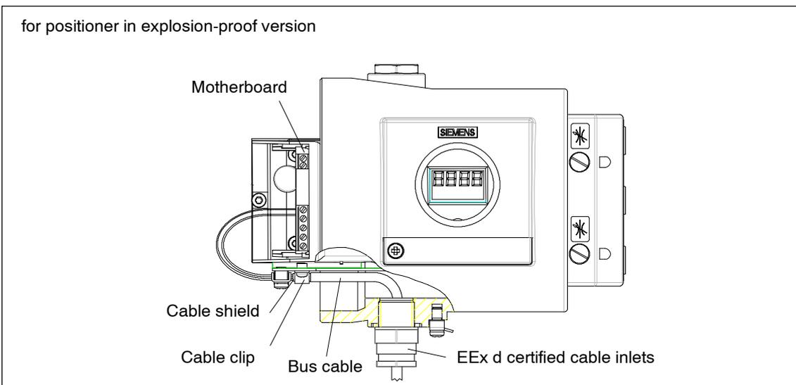
Figure 3-15 Bus cable connection for positioner in explosion-proof version
