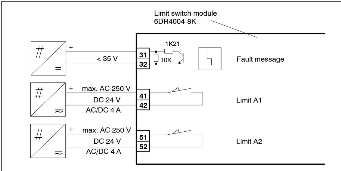
Figure 3-21 Mechanical limit switch module 6DR4004-8K, **non Ex**
