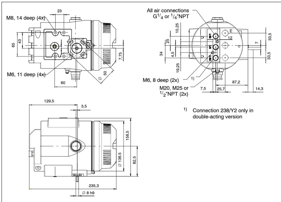
Figure 3-4 Dimensional drawing for positioner with metal housing in explosion-proof version 6DR5xx5
