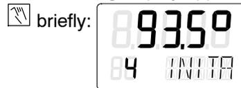
To exit the **Configuration** mode, press the operation mode key
