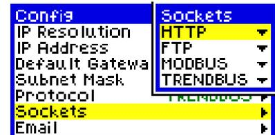
**Socket** number should not need to change. This must only be changed for networking by advanced users. The socket numbers are set according to each type of socket.
