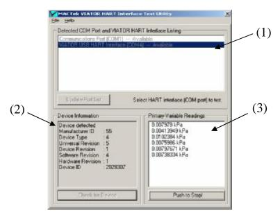
After connecting a HART Device (page 3: **Connecting to a HART Device)**, start VIATORCheck and the VIATOR Interface will be listed in the top window (1). Clicking on "Check for Device" causes the device to be questioned and its information in to be displayed in window (2). Clicking on "Read Primary Variable" reads and displays the device's primary variable in window (3).
