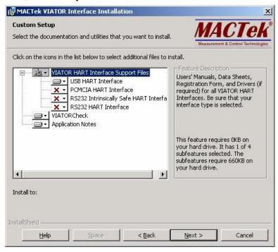
Highlighting an item will display its description and size in the area to the right of the item list. Clicking on the icons will present the option of installing (default) or not installing that item. The USB HART Interface must be selected for the drivers to be installed.
