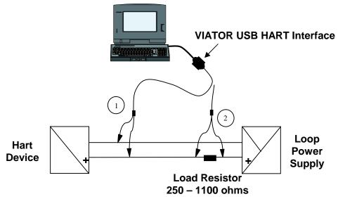
Connect the test clips
