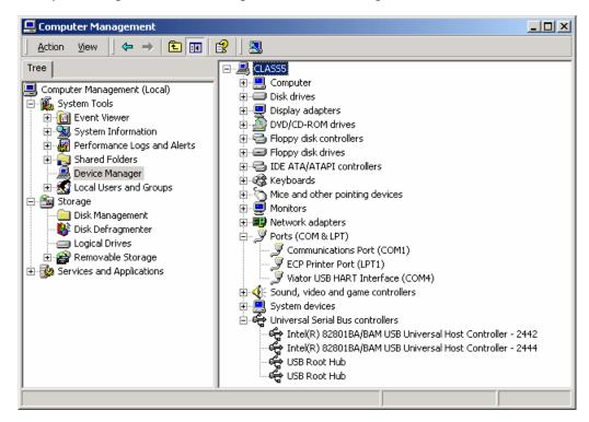
The assigned COM number (in this example COM4) may be different between each host PC and can depend upon which USB socket the Interface is plugged into.
