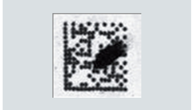
Damaged surface of the marking or part
