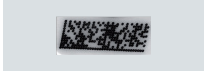
Incorrect overall geometry of the marking
