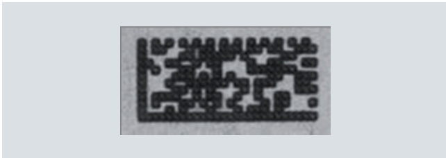
Incorrect or non-uniform cell size in the marking
