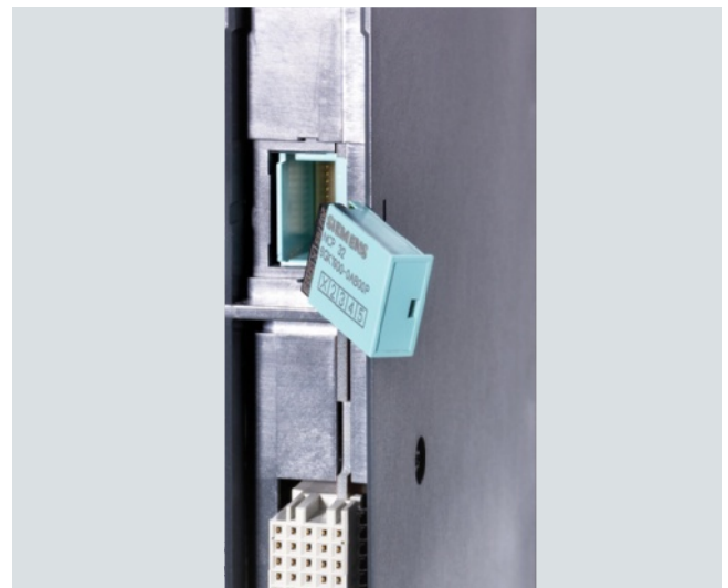
The C-PLUG is plugged into the rear of the CP 443-1 Advanced
