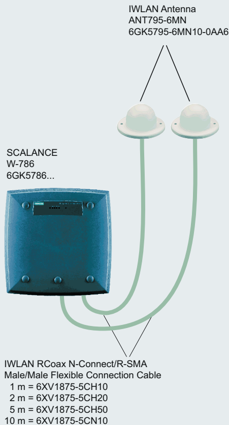
Access Point SCALANCE W-786 with remote antenna
