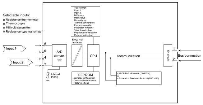
Figure 3-2 Function block diagram SITRANS TH400
