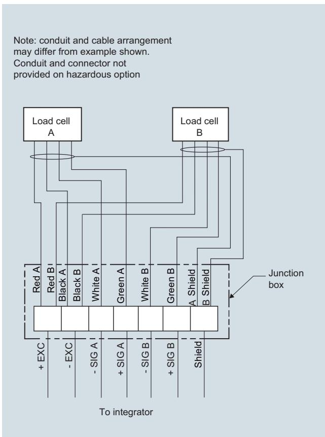
WF200 and WF250 connections
