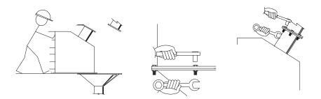
Install the sensing plate. Refer to the appropriate instruction manuals for levelling, sensing plate installation and integrator interconnection instructions.
