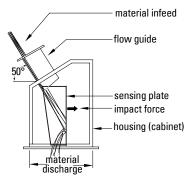
The flowmeter load cells output signals are processed by the flowmeter integrator (ordered separately) to:
