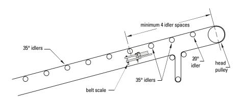
**Recommendation:** On conveyors with 45° trough idlers throughout, a minimum of two 45°, one 35°, and one 20° retreat idlers must be located between the scale and the head pulley.
