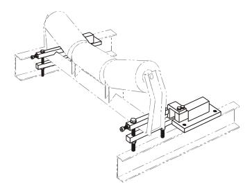
An idler (supplied and installed by customer), test weight bracket and test weights (ordered separately) complete the weighing assembly. The MBS load cells provide an electric signal proportional to load, which is fed to the integrator. Weighing occurs without interrupting the process or affecting the process material.
