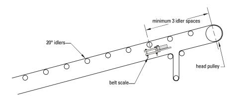
**Recommendation:** On conveyors with  $35^{\circ}$  trough idlers throughout, a minimum of two  $35^{\circ}$  and one  $20^{\circ}$  retreat idlers must be located between the scale and the head pulley.
