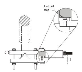
**Note:** The load cell stop is set at the factory to allow the load cell to deflect up to 150 % of its design load. Maximum gap approximately 0.8 mm (0.030").
