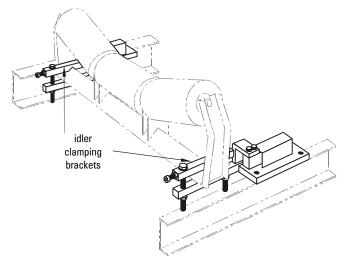
6. The idlers in the weighing area (A2 through R2) must be aligned to and square to the stringers, and levelled to a common reference such as a string or wire (refer to subsequent figures). Ensure that the reference is taut (no sagging). If necessary, shim these idlers to be in line with the reference.
