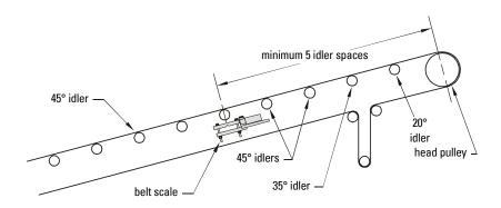
**Recommendation:** The vertical displacement of the head pulley relative to the adjacent retreat idler is normally in excess of that which is acceptable for belt scale installations. It is suggested that when locating the scale close to the head pulley, a maximum of 13 mm (½") vertical displacement between the top of the head pulley and the top of the center roll of the adjacent roll be allowed.
