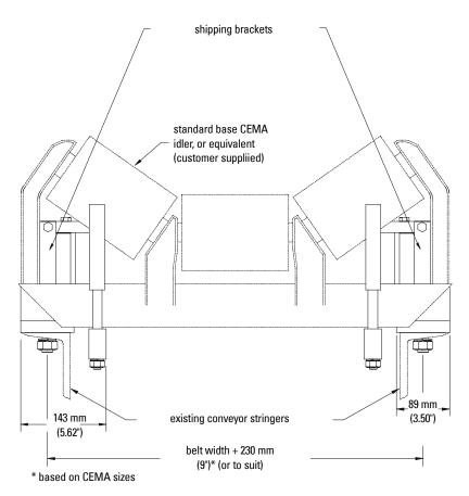
The ideal placement of the Milltronics Universal Scale depends on the conveyor system. This section provides guidelines to determine MUS placement.
