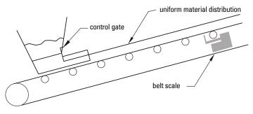
Note: Ensure steady and uniform material loading to the belt at or near the same speed as the conveyor belt. The installation of a material feed control gate or similar device improves uniform flow of material.
