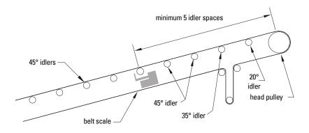
**Recommendation:** The vertical displacement of the head pulley relative to the adjacent retreat idler is normally in excess of that which is acceptable for belt scale installations. It is suggested that when locating the scale close to the head pulley, a maximum of 13mm ( $\frac{1}{2}$ ") vertical displacement between the top of the head pulley and the top of the center roll of the adjacent roll be allowed.
