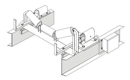
An idler (supplied and installed by customer) and test weights (ordered separately) complete the weighing assembly. The MUS load cells provide an electric signal proportional to load, which is fed to the integrator. Weighing occurs without interrupting the process or affecting the process material.
