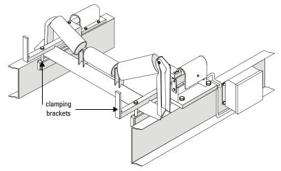
6. The idlers in the weighing area (A2 through R2) must be aligned to and square to the stringers, and levelled to a common reference such as a string or wire (refer to subsequent figures). Ensure that the reference is taut (no sagging). If necessary, shim these idlers to be in line with the reference.
