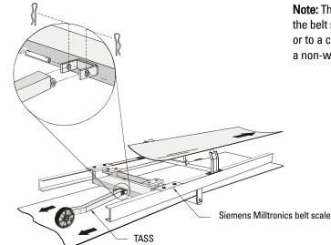
**Note:** The TASS can be mounted to the belt scale static beam as shown, or to a conveyor cross member or to a non-weighing idler frame.
