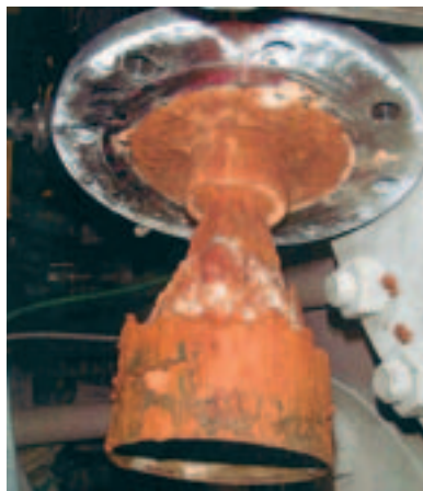
Reliable radar level measurement during titanium dioxide production – despite extreme deposits on the horn antenna
