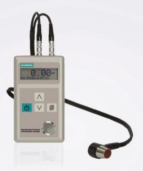
The easy-to-use digital ultrasonic pipe wall thickness gauge from Siemens is an indispensable tool in accurate clamp-on ultrasonic flow measurement. For a flowmeter to measure correctly it needs to know the exact wall thickness of the pipe it is measuring on. Since even the smallest miscalculation can have a
