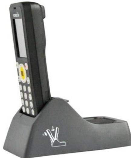
Figure 4-2 RF650M mobile reader in the charging station
