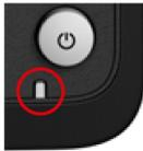
Figure 4-4 LED display of the reader
