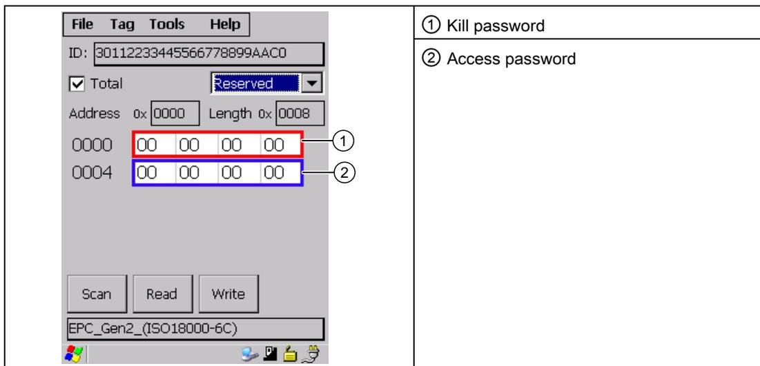
For further information on the detailed structure of the different areas, see "EPCglobal-Specification for RFID Interface" (EPCTM Radio-Frequency Identity Protocols Class-1 Generation-2 UHF RFID Protocol for Communications at 860 MHz - 960 MHz, Version 1.0.9)
