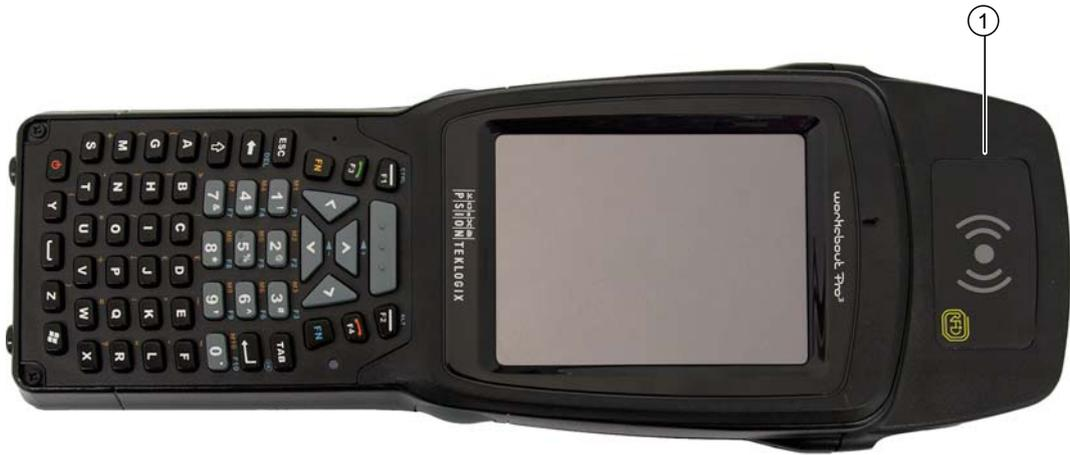
Figure 3-1 Read head with antenna
