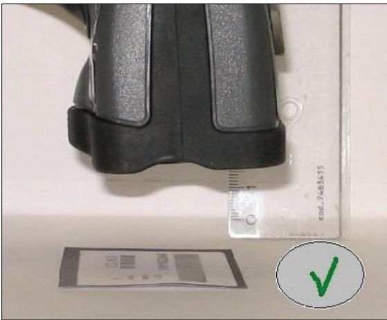
Correct – Move in steadily with front of imager parallel to surface.
