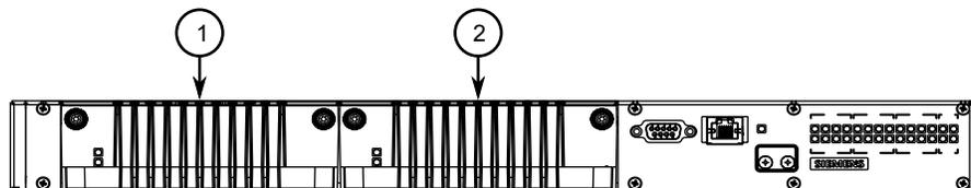
**Figure 7: Power Module Slots**
