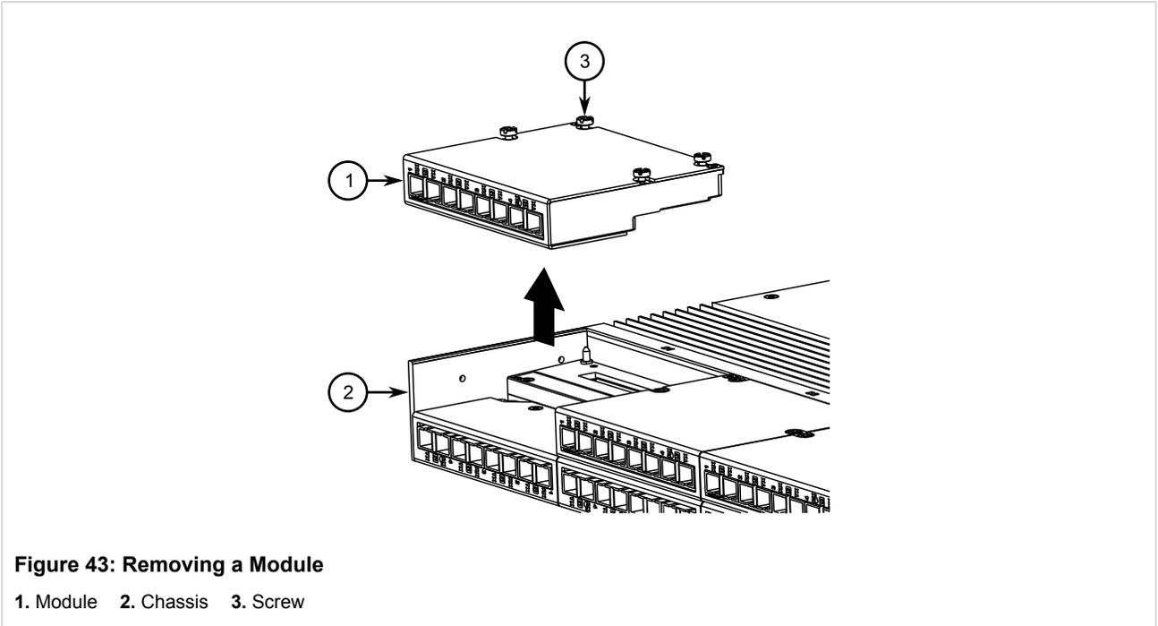
5. Install a new module or a blank module (to prevent the ingress of dust and dirt). For more information, refer to [Section 3.5.1, "Installing Modules"](#).
