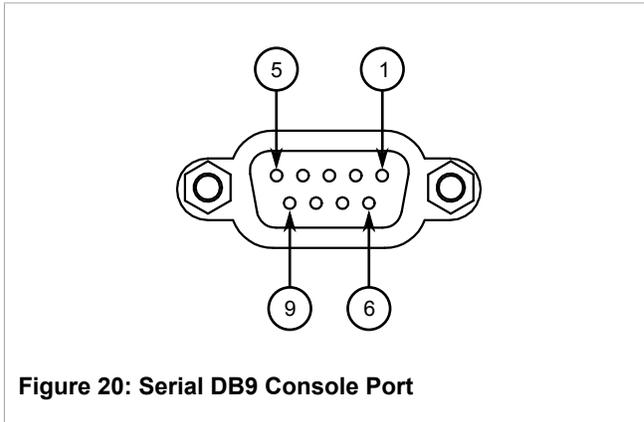
**Figure 20: Serial DB9 Console Port**
