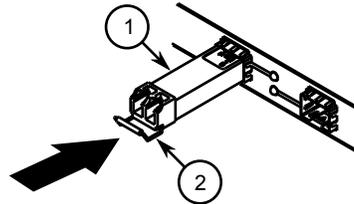
**Figure 39: Installing an SFP Optical Port (Typical)**
