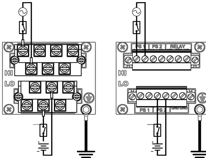
Figure 16: High AC/DC Power Supply and Low DC Power Supply
