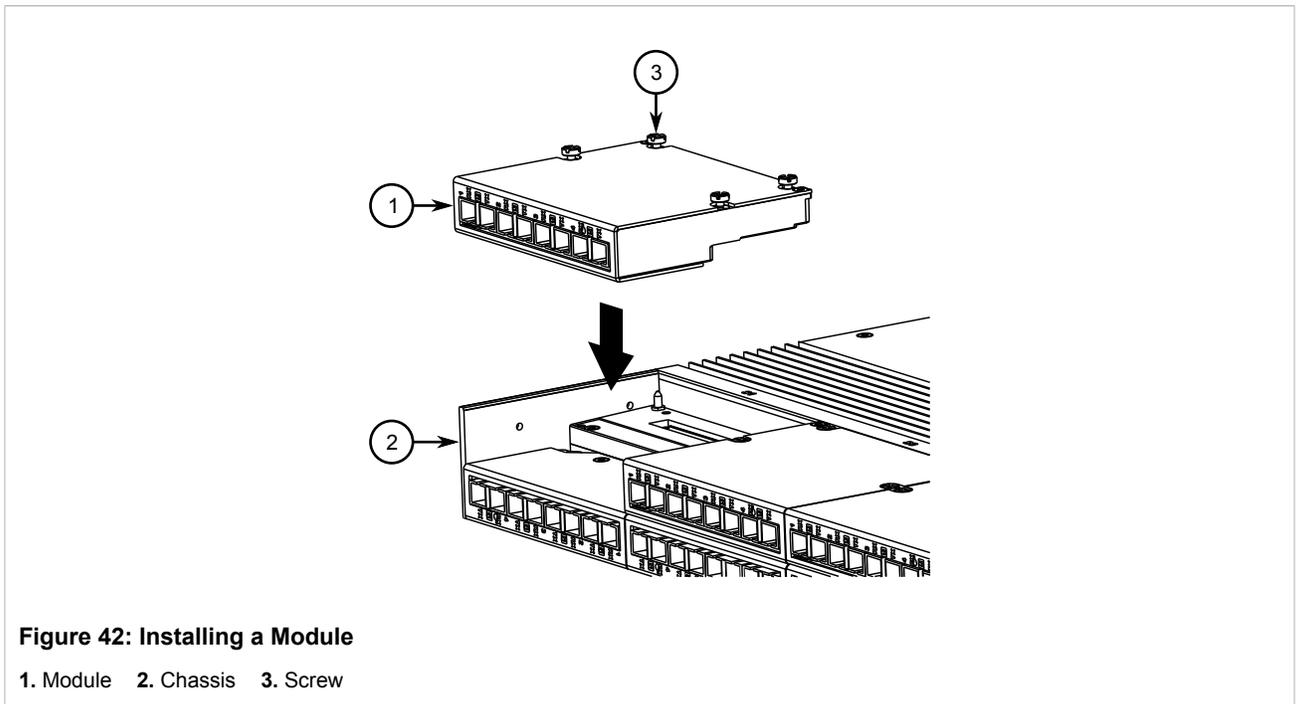
5. Tighten the screws to secure the module.
