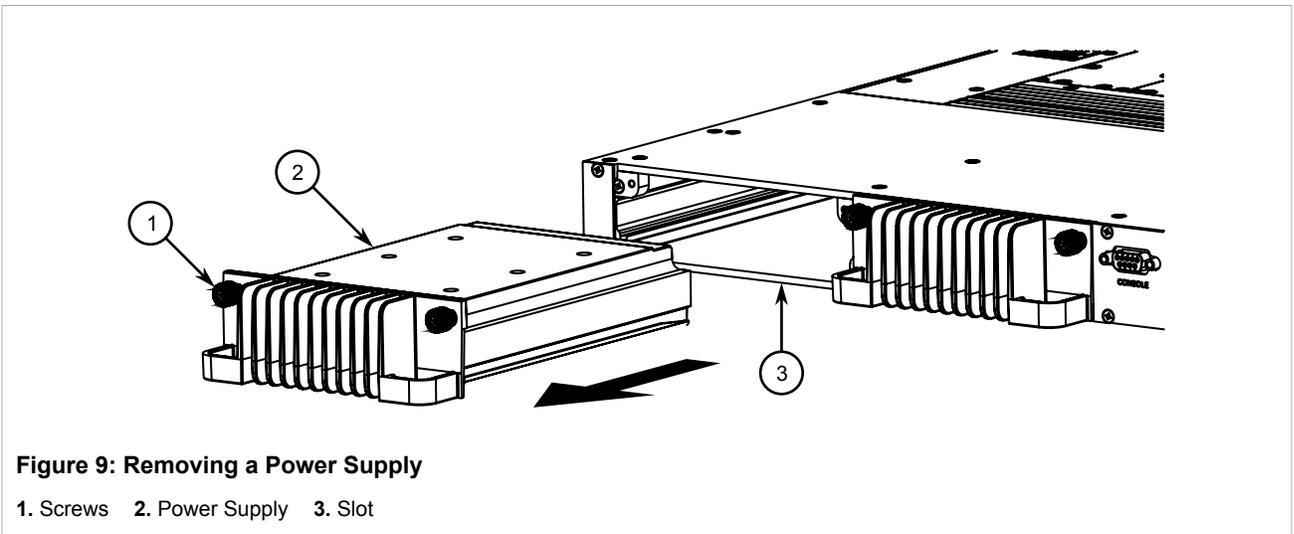
3. Install the blank power module assembly into the empty slot to prevent the ingress of dust and dirt.
