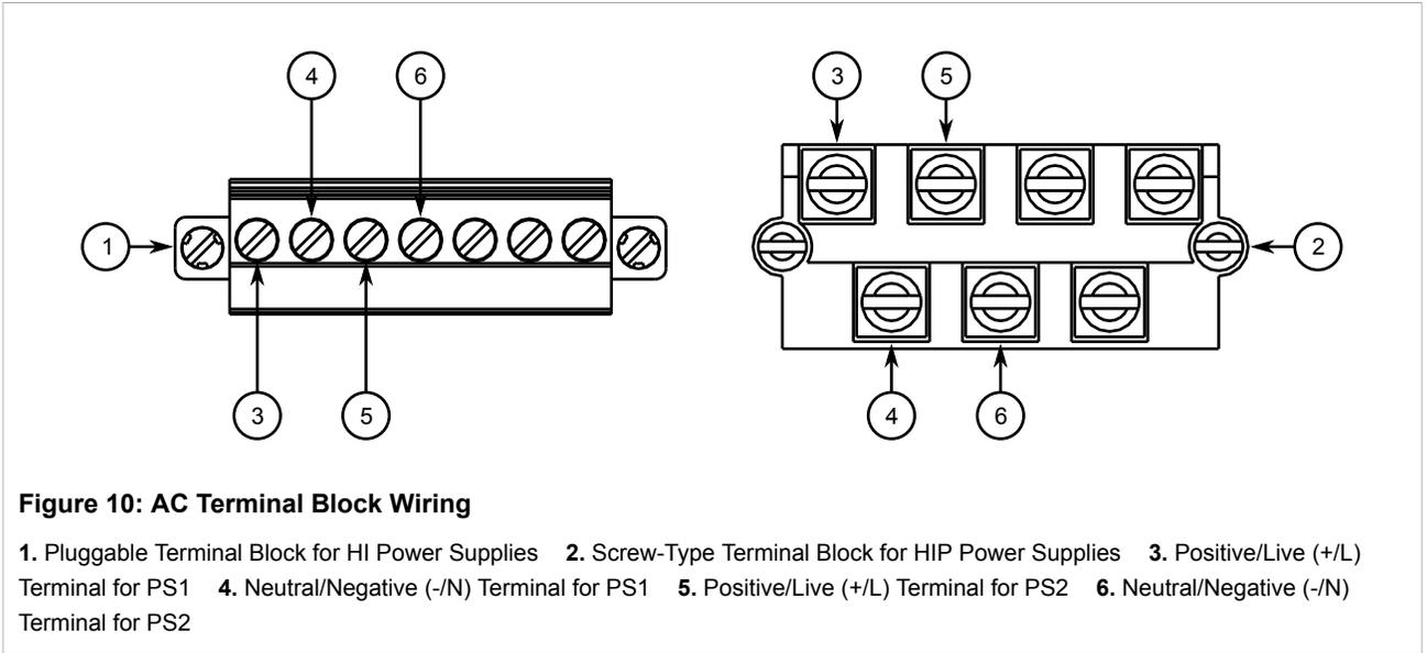
2. Connect the negative wire from the power source to the neutral/negative (-/N) terminal on the terminal block.
