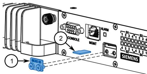
**Figure 19: Inserting/Removing a MicroSD Card**
