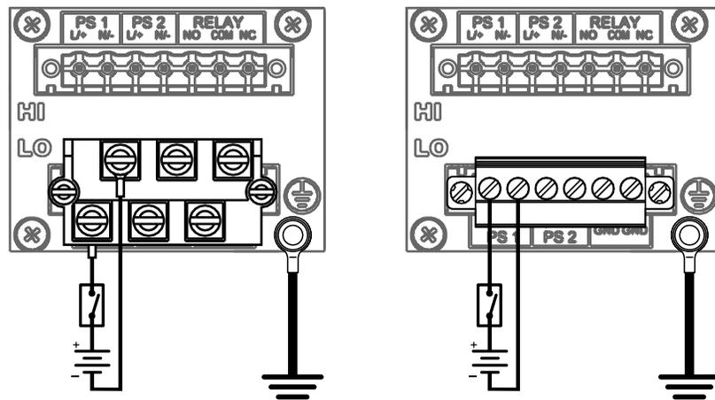
Figure 13: Single Low DC Power Supply
