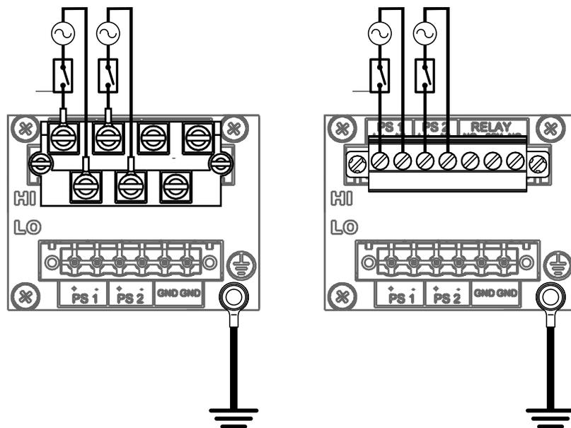
Figure 14: Dual High AC/DC Power Supply
