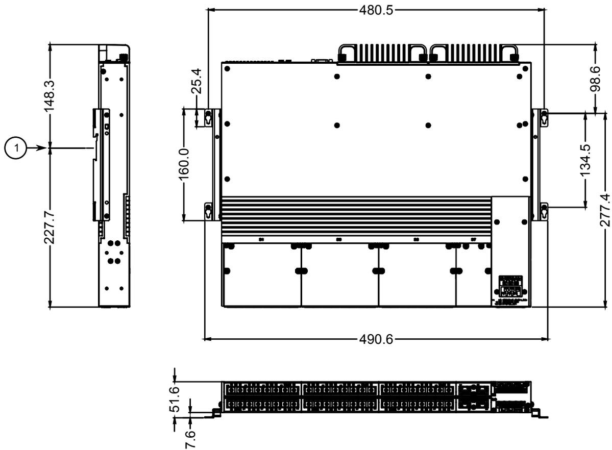
**Figure 46: Panel and Din Rail Mount Dimensions**
