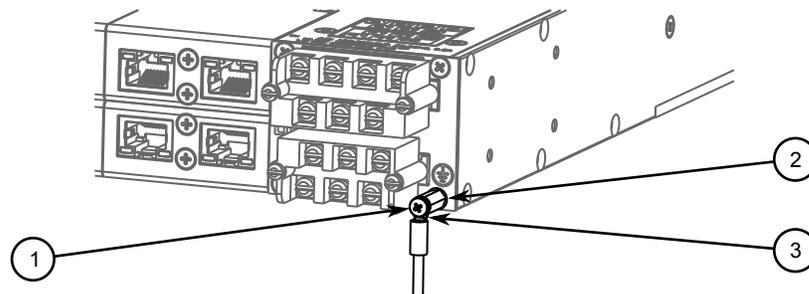
**Figure 18: Chassis Ground Connection**
