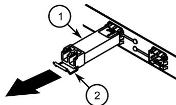
**Figure 40: Removing an SFP Optical Port (Typical)**
