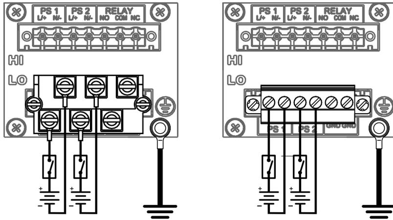
Figure 15: Dual Low DC Power Supply
