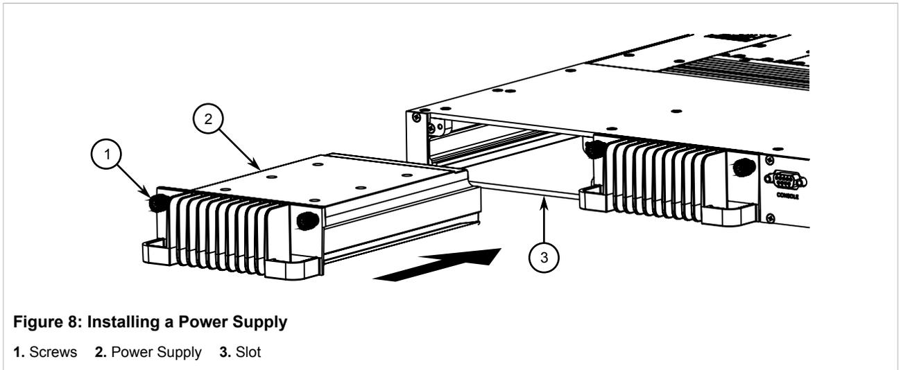
3. Hand-tighten the screws to secure the power supply.
