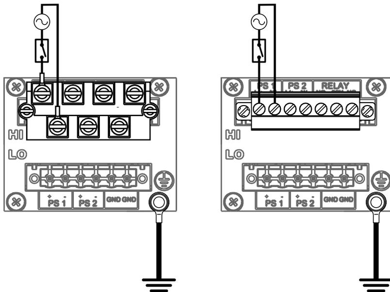
**Figure 12: Single High AC/DC Power Supply**
