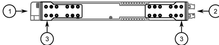
**Figure 4: Rack Mount Adapters**
