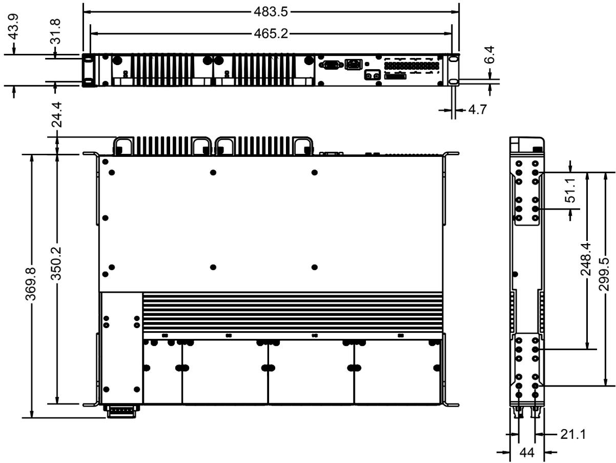
Figure 45: Rack Mount Dimensions
