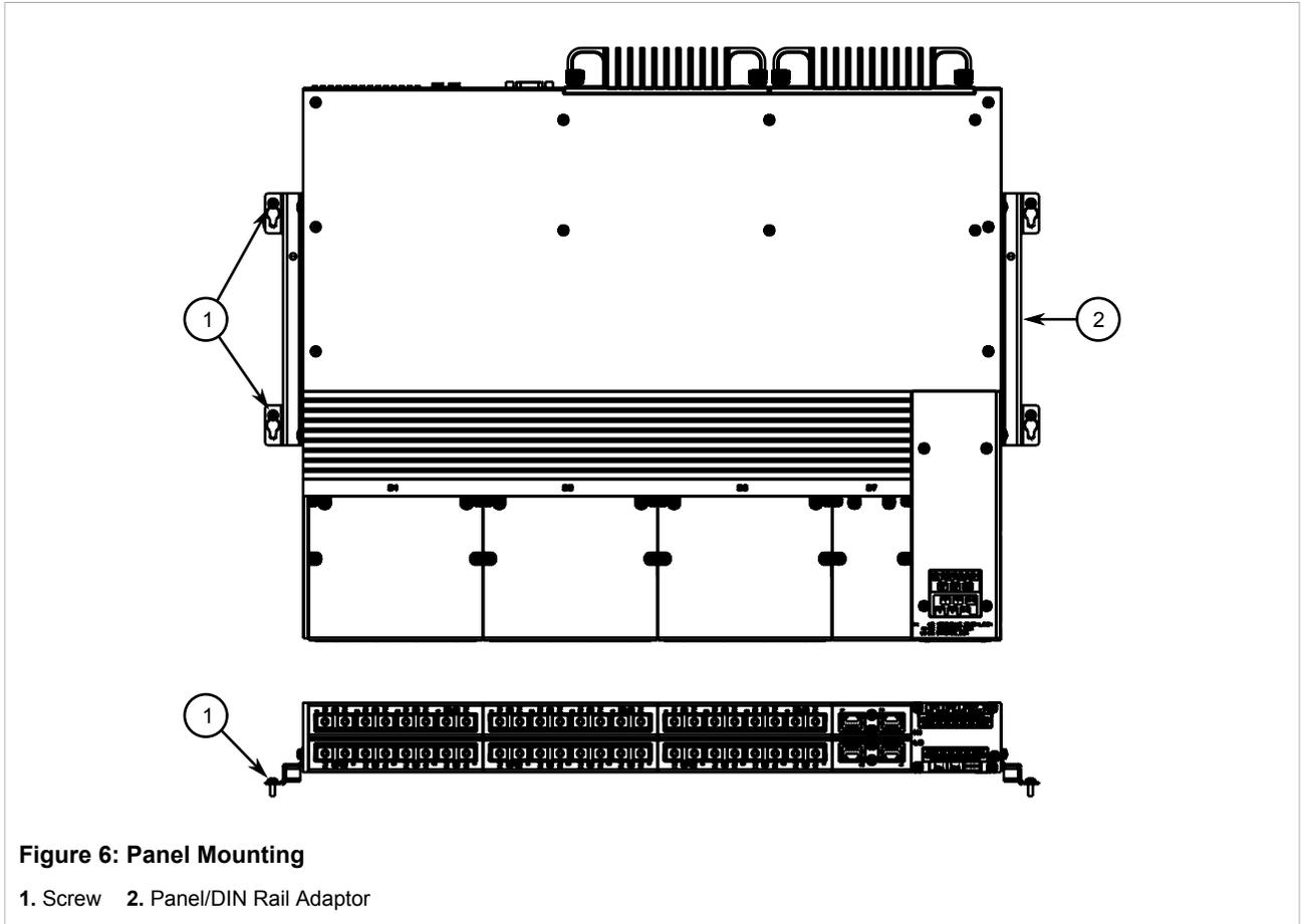
2. Install the supplied screws to secure the adaptors to the panel.
