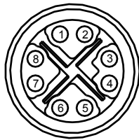
Figure 26: 8-Pin M12 X-Coded Ethernet Port Pin Configuration
