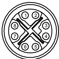
Figure 23: 8-Pin M12 X-Coded Ethernet Port Pin Configuration
