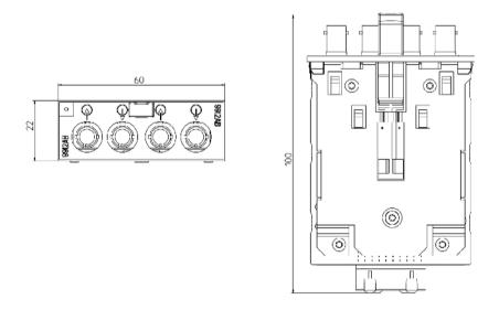
Image 5-3 MM900 dimension drawing 3: BFOC ports
