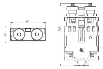
Image 5-6 MM900 dimension drawing 6: M12 ports electrical
