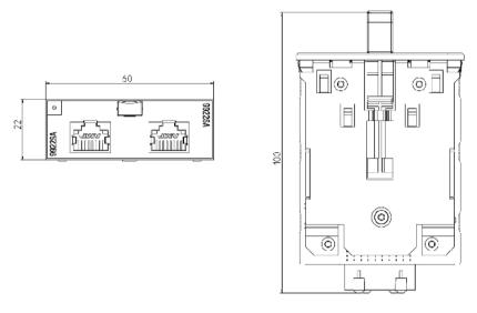
Image 5-2 MM900 dimension drawing 2: Electrical RJ-45 ports without securing collar
