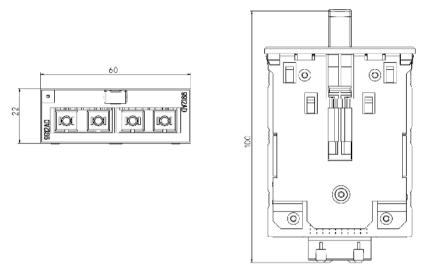
Image 5-4 MM900 dimension drawing 4: Optical SC ports
