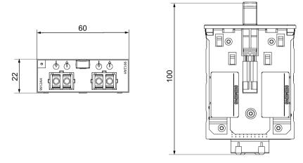
Image 5-7 MM900 dimension drawing 7: SC RJ ports optical
