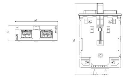
Image 5-5 MM900 dimension drawing 5: SFP media module
