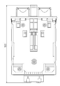
Image 5-1 MM900 dimension drawing 1: Electrical RJ-45 ports with securing collar
