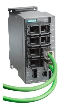
Figure 5-2 Plugging in the IE FC RJ45 Plug 180
