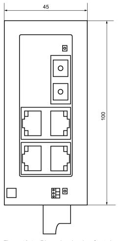
Figure 10-1 Dimension drawing, front view (example: SCALANCE XB004-1)
