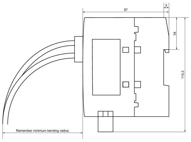
Figure 10-2 Dimension drawing, side view (example: SCALANCE XB004-1)
