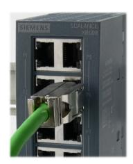
Figure 6-2 Plugging in the IE FC RJ45 Plug 180
