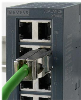
Figure 5-2 Plugging in the IE FC RJ45 Plug 180
