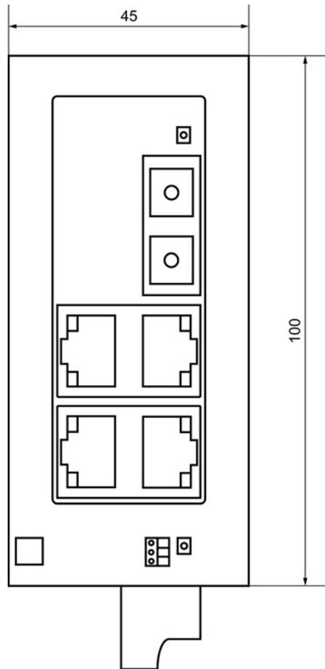
Figure 9-1 Dimension drawing, front view (example: SCALANCE XB004-1)
