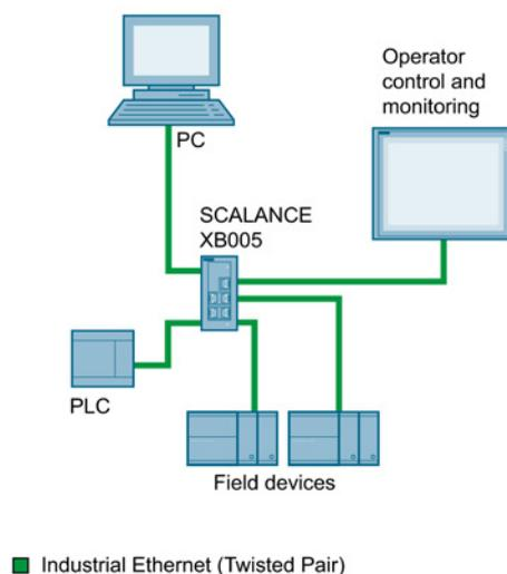
Figure 2-1 Example of an electrical star topology with SCALANCE XB005
