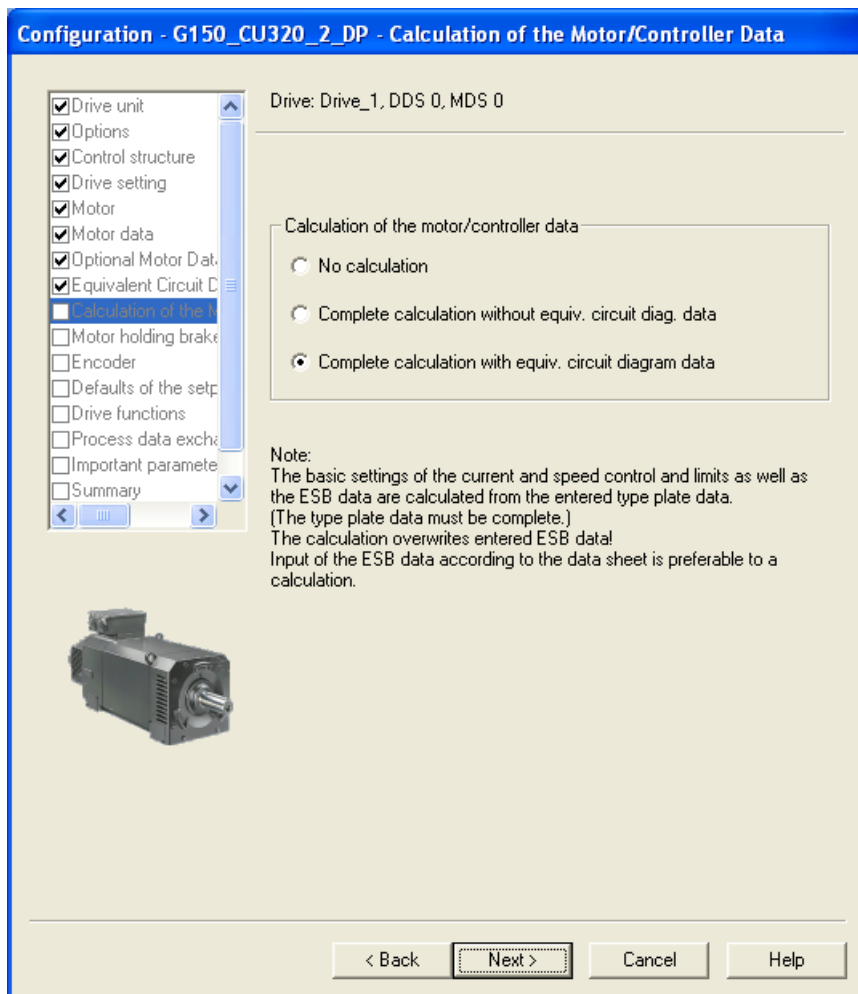
Figure 5-21 Calculating the motor/controller data
