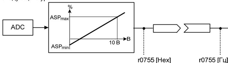
$$r0755 \text{ [Гц]} = \frac{r0755 \text{ [Hex]}}{4000 \text{ [Hex]}} \cdot P2000 \cdot \frac{\max(|ASP_{\max}|, |ASP_{\min}|)}{100\%}$$
