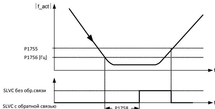
$$P1756 \text{ [Гц]} = P1755 \text{ [Гц]} \cdot \frac{P1756 \text{ [%]}}{100 \text{ [%]}}$$
