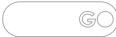
Figure B.3: *Go* tool used in the validating procedure (1.5 mm thickness)
