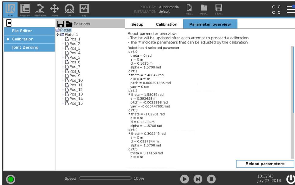
Figure 1.10: The identified parameters are displayed in the **Parameter overview**.
