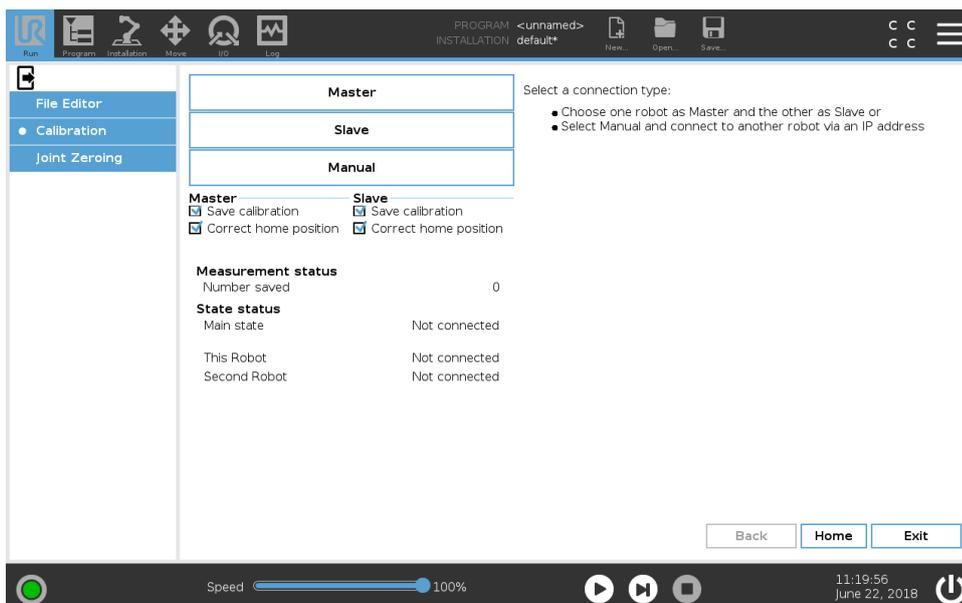
Figure 2.9: Network options in Dual Robot Calibration.
