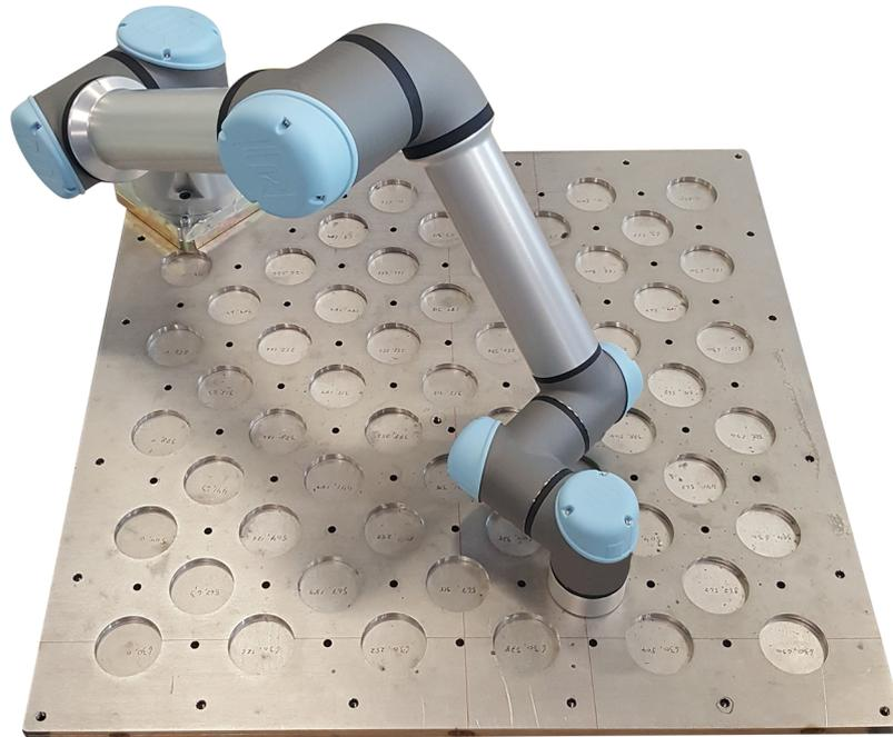
Figure 1.1: Robot mounted on a plate during Plate Calibration.
