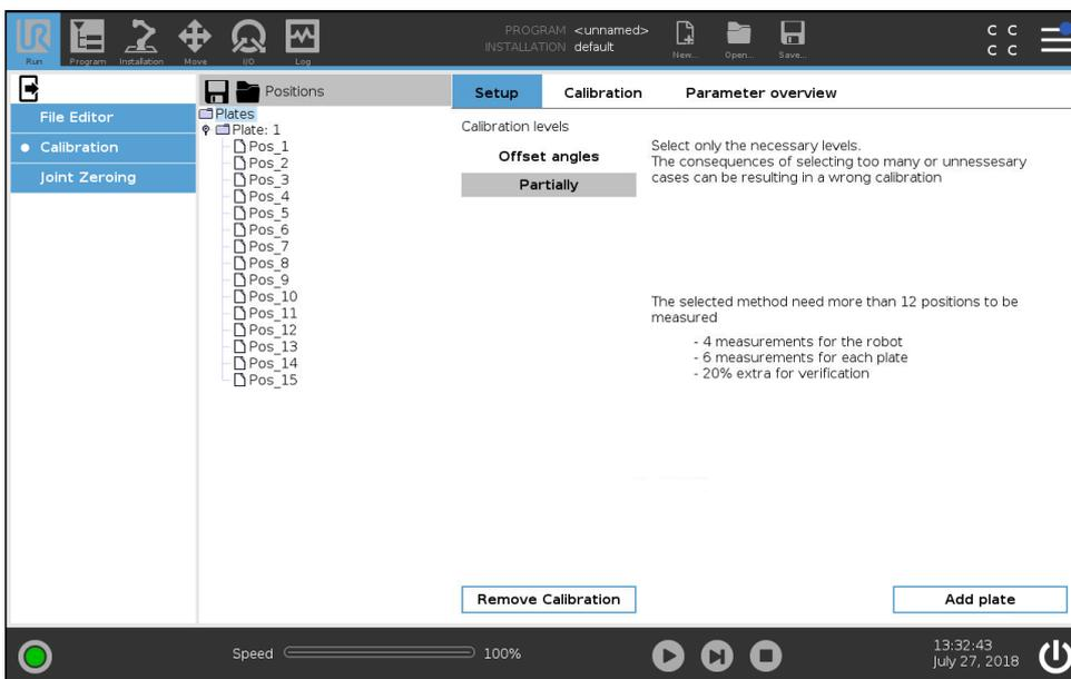
Figure 1.8: Select the top of the tree item on the left to be able to select the level of calibration, then select the Calibration Tab and press **Make Calibration** to start the calibration.
