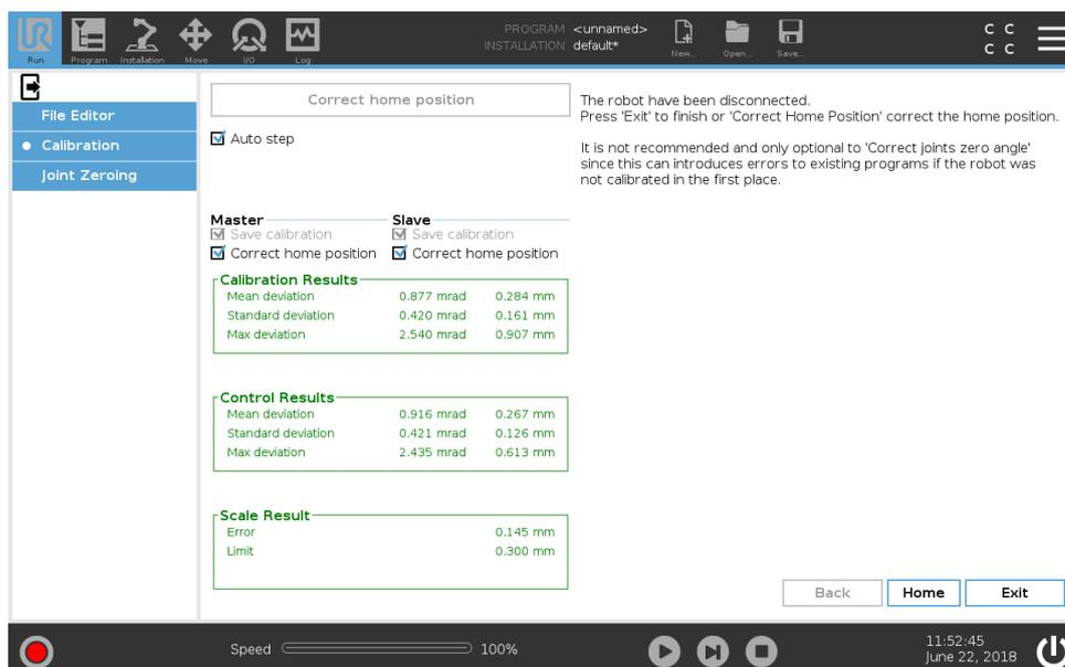
Figure 2.24: Successful calibration
