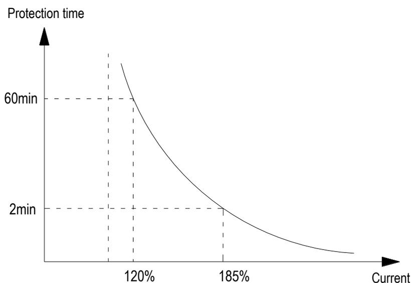
In the above figure, the horizontal axis is the current entering the protection curve, that is, the percentage of the rated current of the motor. The calculation formula is: horizontal axis current = (motor actual current / motor overload protection coefficient) × 100%, so increasing F10.30 can improve the motor Overload capability.
