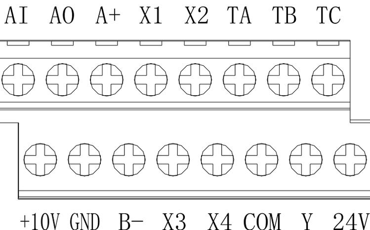
7.5kW-22kW Control circuit terminal arrangement
