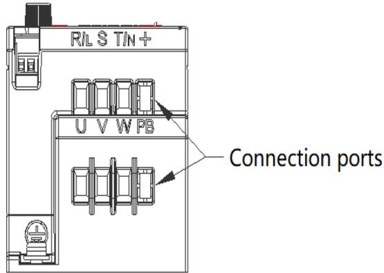
0.4kW-5.5kW Terminal arrangement
