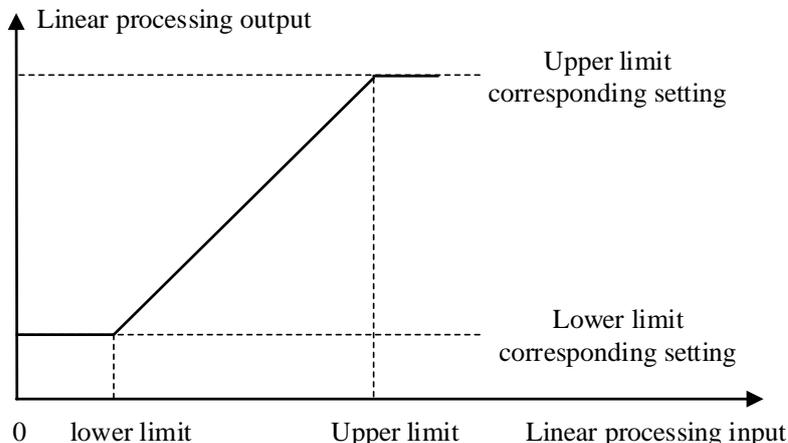
Schematic diagram of linear processing of PUL input frequency
