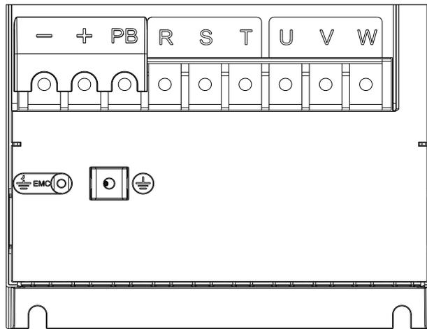
7.5kW-22kW Terminal arrangement
