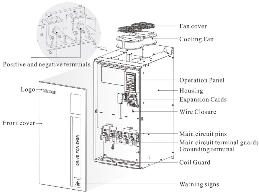
Among them, the + - terminal is located on the left side of the inverter under the fixed small iron plate (as shown above, this small iron plate can be easily removed).
