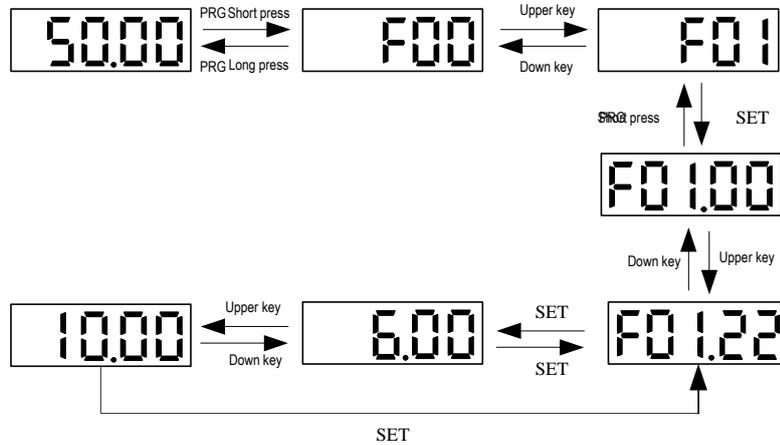
**Note:** Use the keypad shift buttons to quickly select the Led "00", Led "000" and Led "0000" of parameter values for modification.
