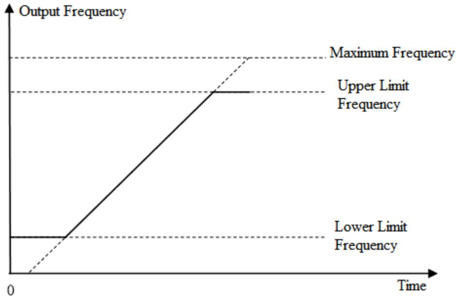
Diagram of Relationship between Maximum Frequency, Upper Frequency Limit and Lower Frequency Limit
