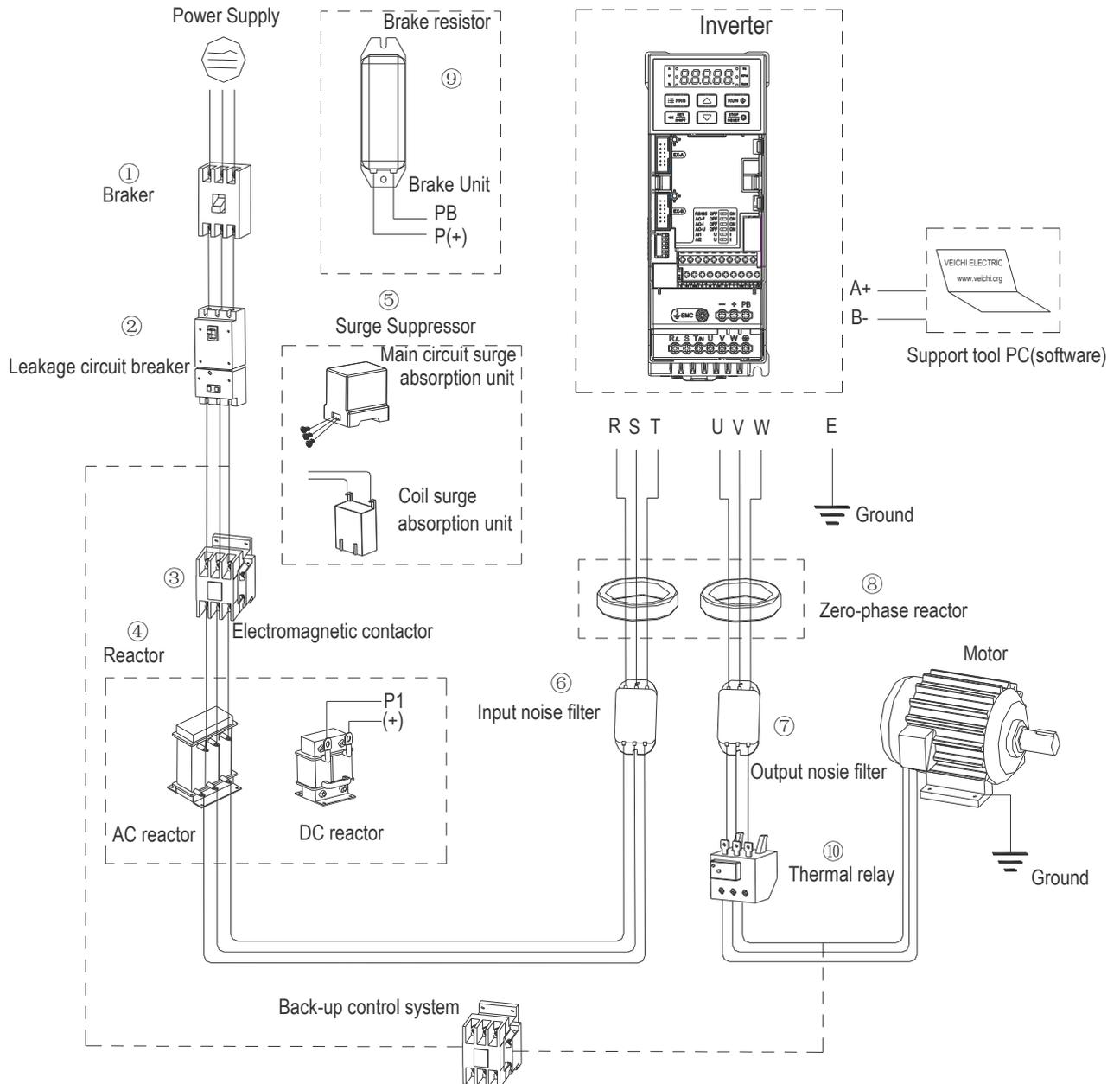
Figure 9-1: Connection block diagram of external devices
