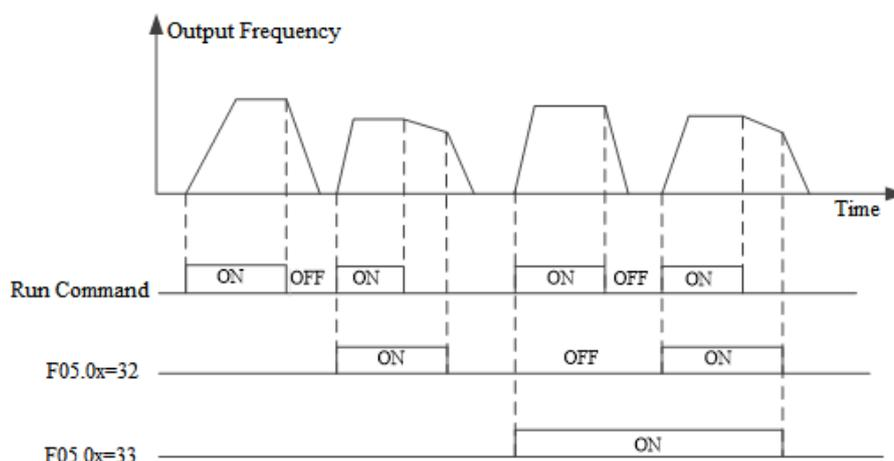
Time Sequence Diagram of Acceleration/Deceleration Time
