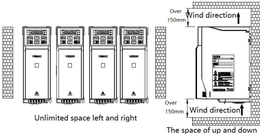
Figure 3-3: Inverter installation space requirements
