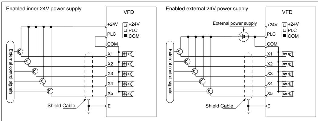
Wiring method of NPN characteristic transistor:
