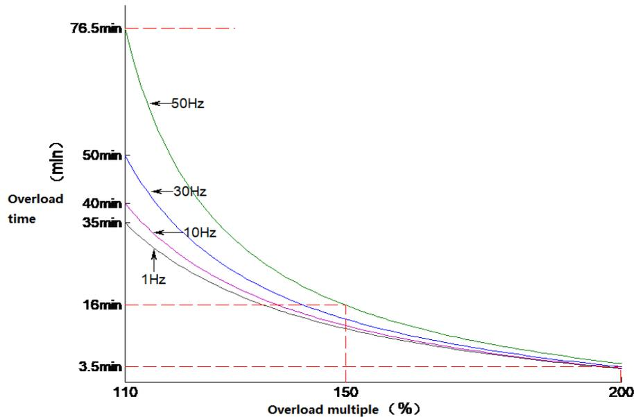
**Note:** Users need to set the industrial control according to the actual condition of the motor, and set the values of F10.55~F10.59 correctly, to effectively protect the motor.
