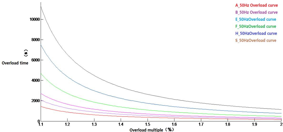
The overload time table of key points of each level at 50 Hz
