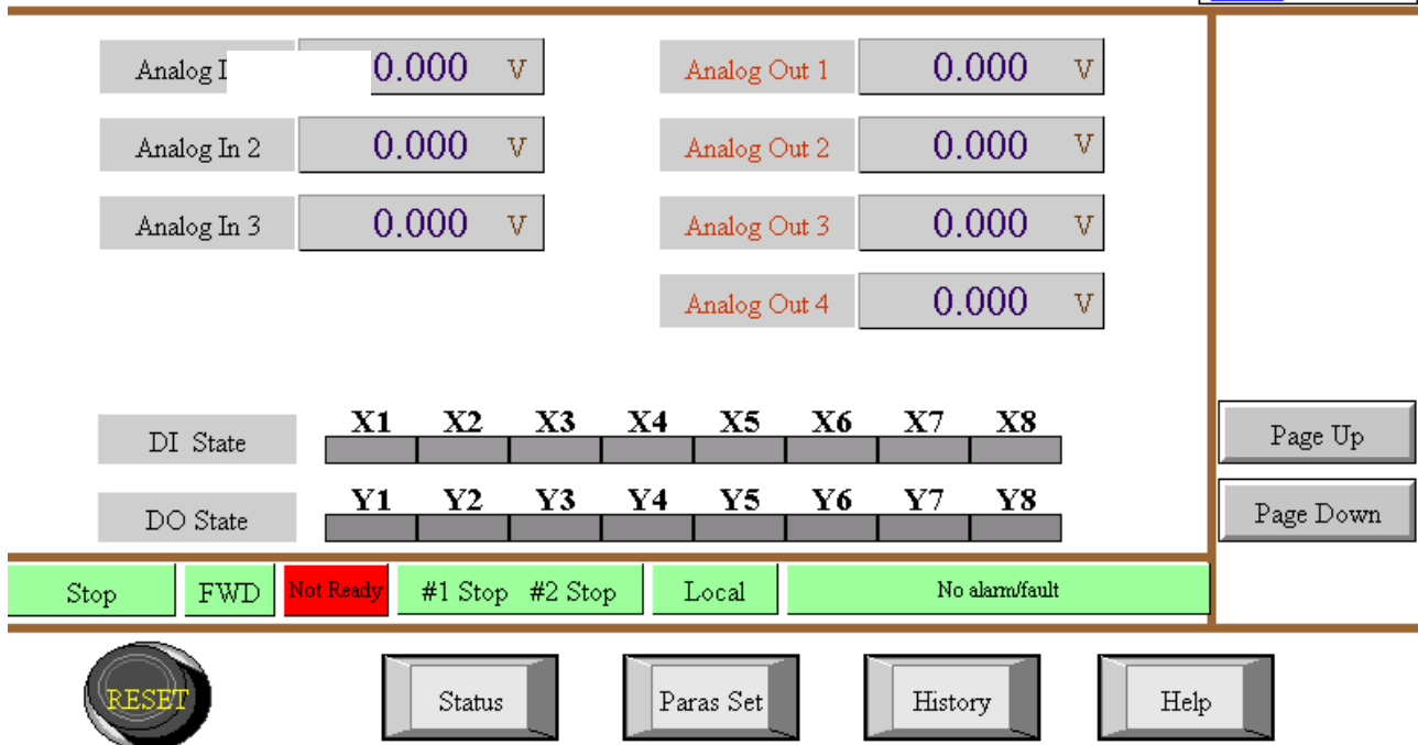
Figure 4.4 The third page of status display of the LCD touch screen of ACH100 high-voltage VFSR system
